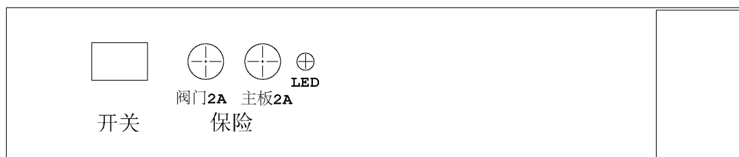
Location of power switch and fuses
